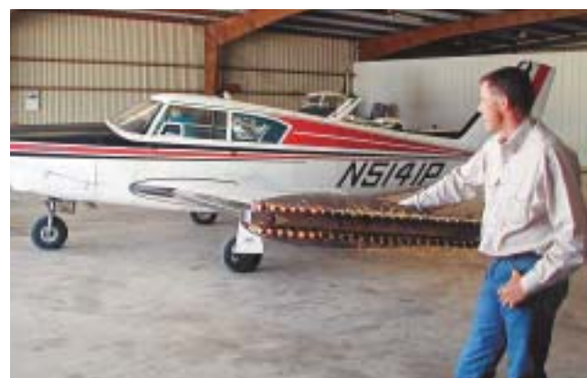
figure 72 - Aircraft fitted with flares for cloud-seeding (Photo courtesy of John Forrest)
